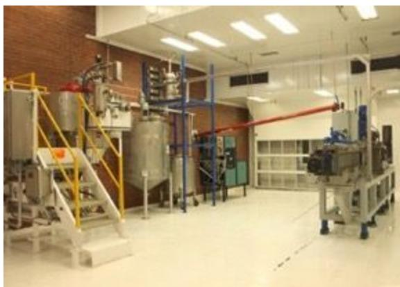
Rather than employing a common industry chemical hydrogenation process using nickel as catalyst, HempSweet has chosen to pursue an industrial-scaled bioreactor fermentation process employing microorganisms to accomplish the final conversion to xylose to xylitol crystal. Similar bioreactors are in broad use and the general technology is well understood and available, but isolating the exact, best pathway to the desired end production at scale requires R&D. Development of
